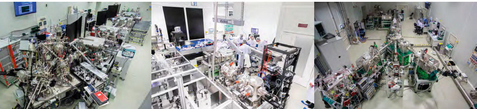
▲ FIG. 1: Selected laser and target areas currently offered to ELI ALPS users (from left to right): the HR (100kHz, 1 mJ) laser in combination with NanoESCA endstation, the Mid Infrared laser (100 kHz, 0.15mJ) with experimental platform (centre) and the SYLOS (1 kHz, 30mJ) driven beamline for attosecond science.
